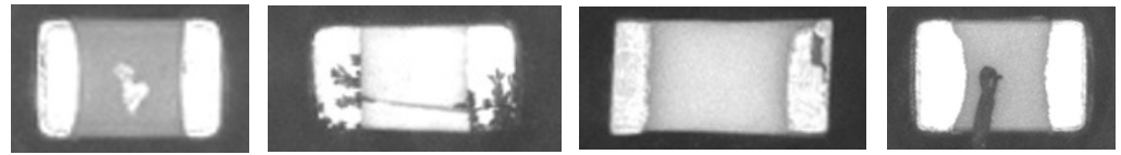
Figure 1. Examples on passive components (left to right): conductive FOD (foreign object debris), corrosion leading to cracks, lead peeling, non-conductive FOD.
