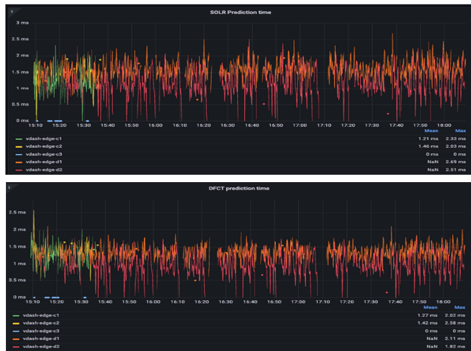
Figure 17. (Top) processing time of the defects detection algorithm, (bottom) processing time of the corrosion detection algorithm, both running in parallel on the same images.
